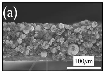
The topology and microstructural interactions determines the power and energy density in three length scales: the electrode thickness level (see (a)), the particle morphology level (see (b)-(d)), and the primary particle level (see (e)).
