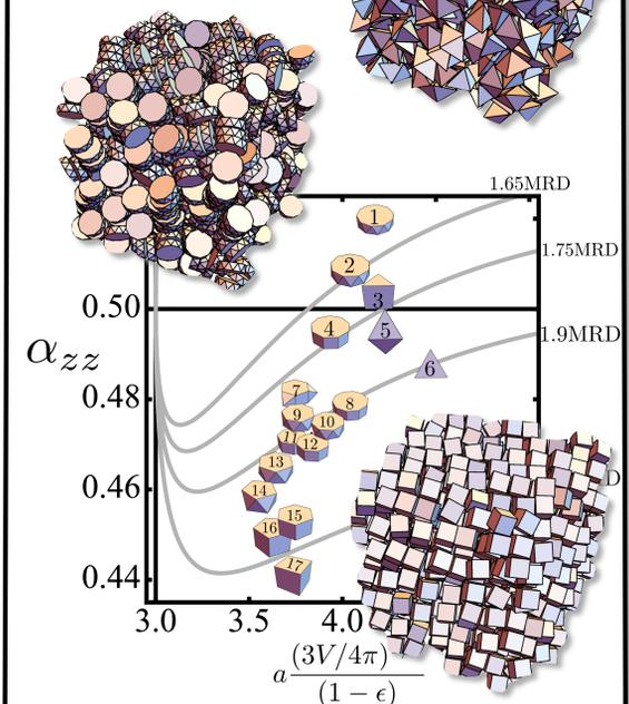
We go well beyond the traditionally used battery models (which treat battery particles as a random distribution of monodispersed spheres; see left side of this poster for examples of real particles), and instead develop and open source software strategies where *the effect of any particle shape on battery performance can be engineered* (see ■ to ▲ below).
