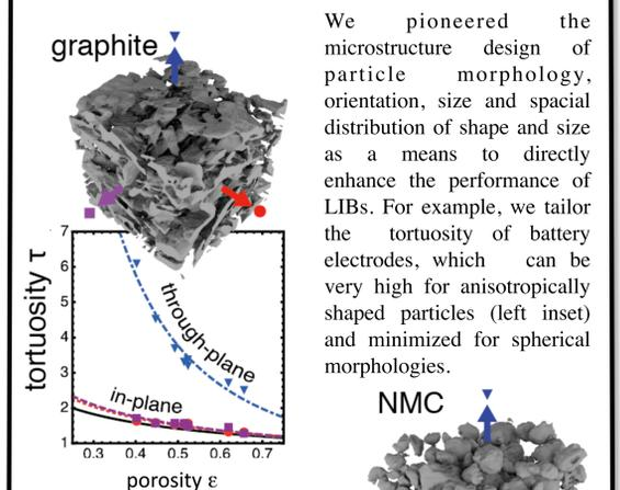
We pioneered the microstructure design of particle morphology, orientation, size and spatial distribution of shape and size as a means to directly enhance the performance of LIBs. For example, we tailor the tortuosity of battery electrodes, which can be very high for anisotropically shaped particles (left inset) and minimized for spherical morphologies.
