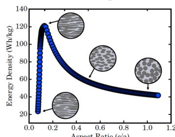
**All roads lead to Rome:** At the end of the day, the aim of the batteries simulation research group is to identify particle chemistries and shapes to optimize the amount of energy stored within an electrode. The example above demonstrates that by combining experimental and simulation data, the energy density can be dramatically increased.
