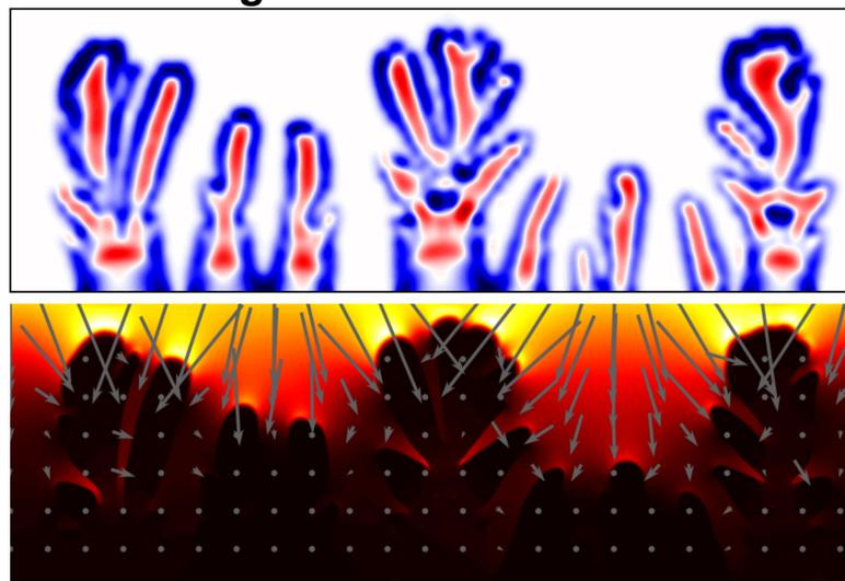
Lithium dendrites (see images above) are electrodeposits that nucleate and grow on battery anodes during recharge (see image in Introduction). Unchecked dendrite growth leads to short circuits and causes catastrophic battery failures. In this project, we develop a unified theoretical framework that delineates growth mechanisms (e.g., tip- and base-controlled growth), as a stepping stone to identify battery fabrication strategies that enable safer, improved devices.
